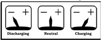
Let's assume the alternator is not working correctly. It is not charging. Your needle goes to discharge. This means it is drawing out energy but not replacing it. Seeing that, you turn off the lights, the air conditioner, the radio, and the windshield wipers. You turn off everything that draws power, and the needle returns to the middle. It is not charging, but it is not discharging, either. You say, "Man, that's living!"
